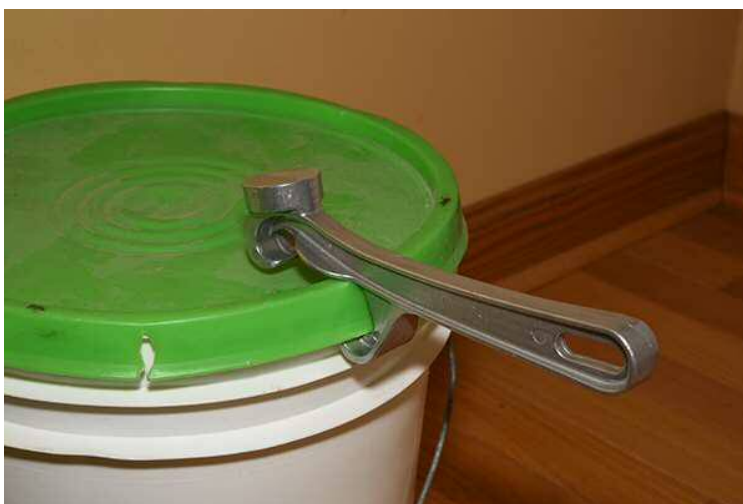
Figure 6.15: Lid Lever – A lid lever can be purchased for under ten dollars. Source: author – [file:\FD-LidOpener01.jpg].
