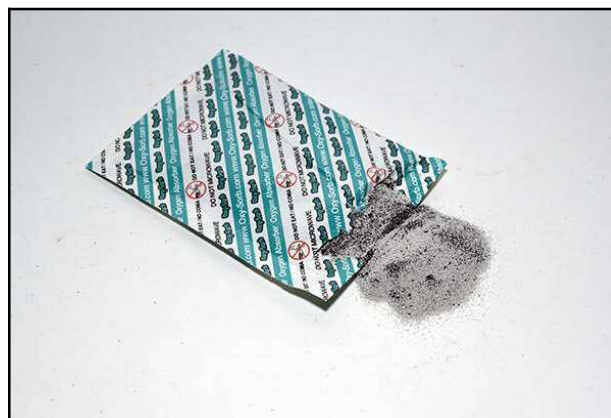
Figure 6.20: Oxygen Absorbers – In the oxygen absorber, the oxygen combines with the iron filings and depletes or removes all the oxygen in the container. Source: author – [file:\FD-OxygenAbsorber.jpg].
