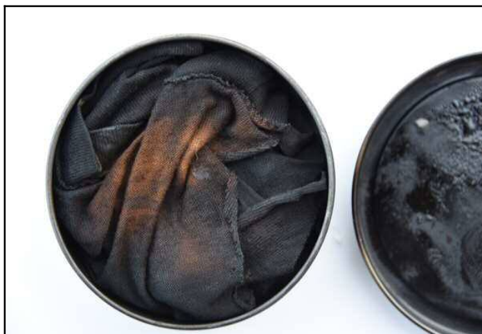
Figure 5.11: Char Cloth – Using the pyrolysis process, the cotton cloth is heated without oxygen. The lighter colored fabric is not yet fully processed. Source: author – [file:\FR-CharCloth03.jpg].
