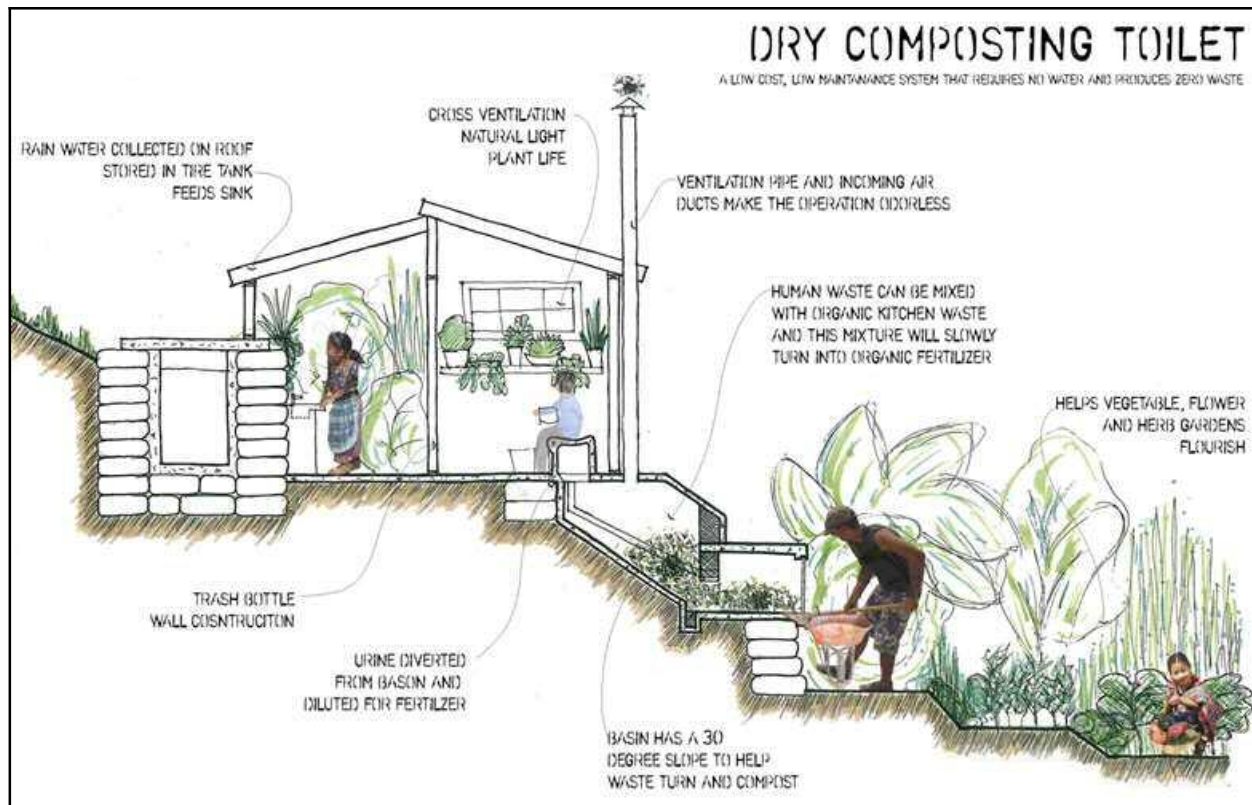
Figure 8.2: Dry Composting Toilet – This scene depicts a dry composting toilet in a third world setting. Source: internet – [file:\DryComposteToilet[120].jpg].
