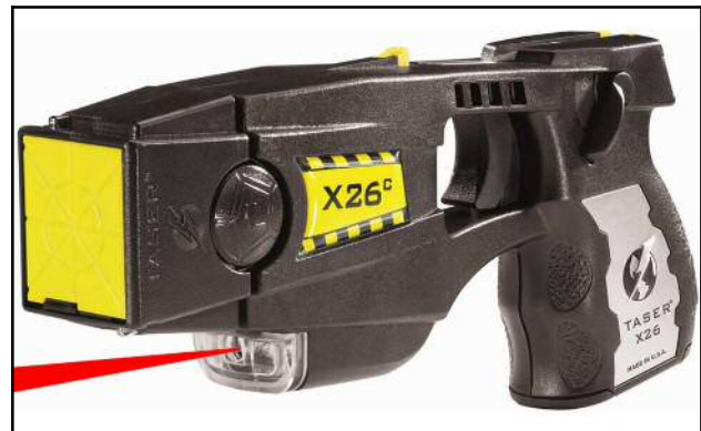
Figure 16.11: Taser ® – The Taser is an electroshock device. Two electrodes are shot toward the victim and the high voltage low amperage current immobilizes the victim. Source: Taser – [file:\Taser[138].jpg]
