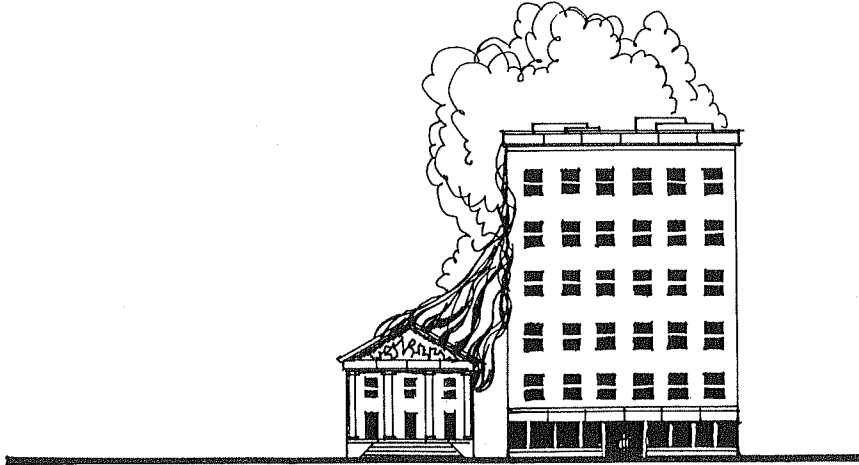
FIRE SPREAD BY CONVECTION
