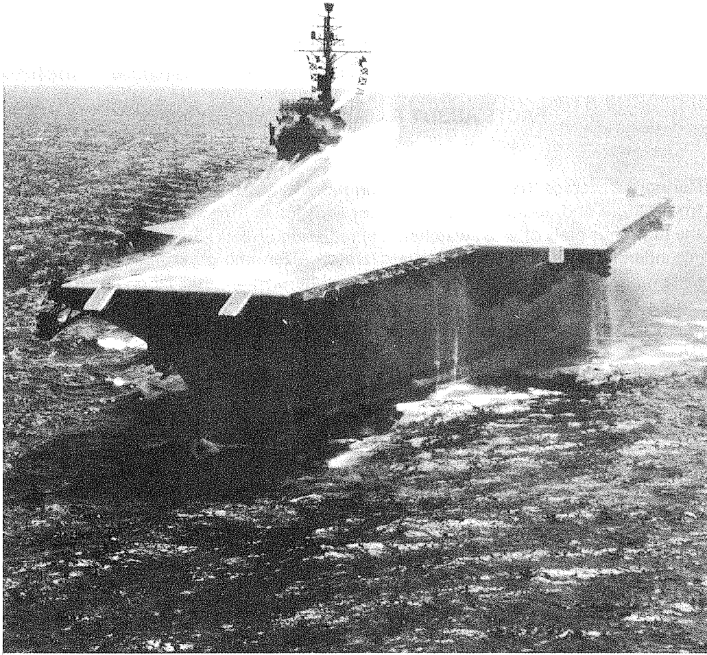
PHOTOGRAPH OF USS KITTY HAWK UNDER WASHDOWN (Courtesy of Office of Chief of Naval Operations)
