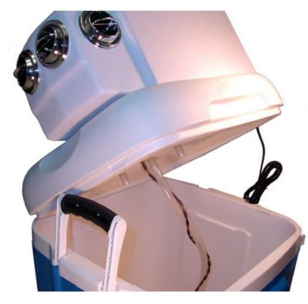
Using powerful Brushless Double Ball Bearing Motors the M300 merely sips power while streaming cool crisp air when & where you need it. This Cooling System has the capacity to produce over 220 cubic feet per minute (cfm) at a velocity of 3,000 feet per minute with a noise level of 59 dBA on high speed. The dBA is slightly higher than our other Swampy models because the motors are operating freely at a higher more efficient R.P.M.
