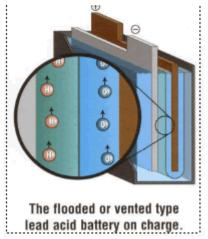
The oldest types of lead acid batteries are flooded cell types. These have been around for decades. The liquid sulfuric acid solution in these batteries has destroyed more than a few sets of clothes and pieces of RV gear. They generate and vent dangerous explosive gases, acid "mist" during charging, corrode their terminals, often-acid damage surrounding surfaces, and require regular watering. They are the least expensive type and therefore are the choice of many RV owners.
