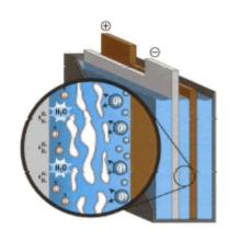
The voids that develop with the nelled electrolyte battery design
