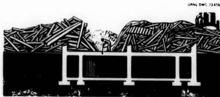
Fig. 123. Making an opening in a roof with a manual drill.
