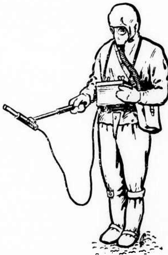
Fig. 99. Determining the radiation level with the DP-5 meter (probe head set in "D" position, at a height of 1 m).
