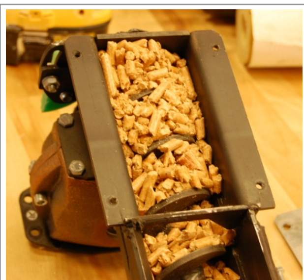
An auger is used to feed pellets into a pellet stove.
