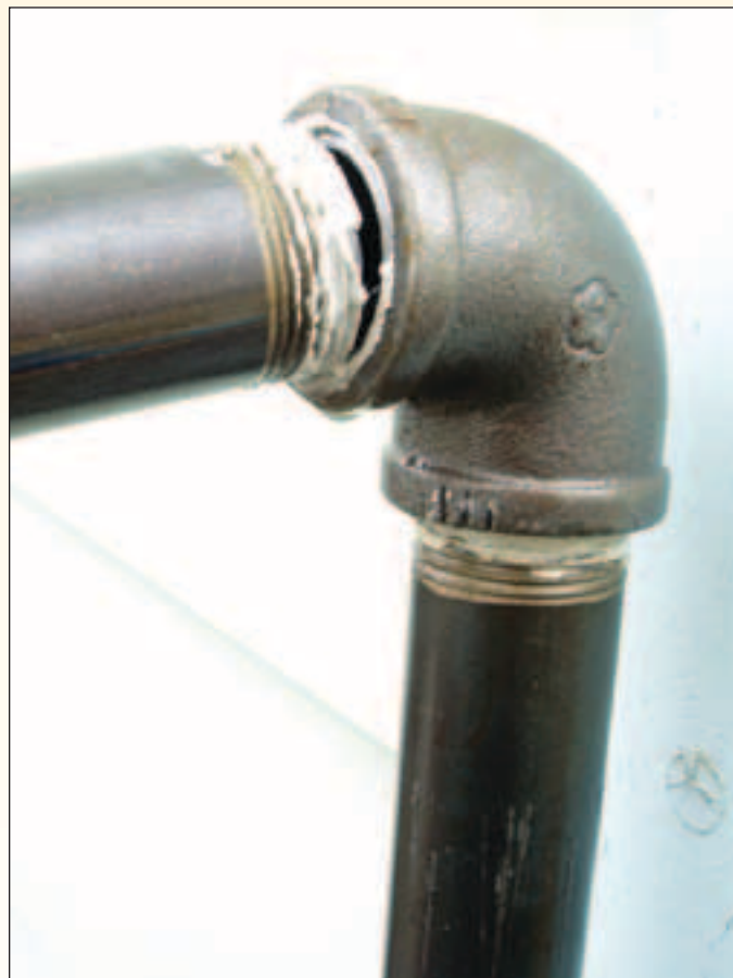
Broken fuel line at elbow due to stress from shifting oil tank.
