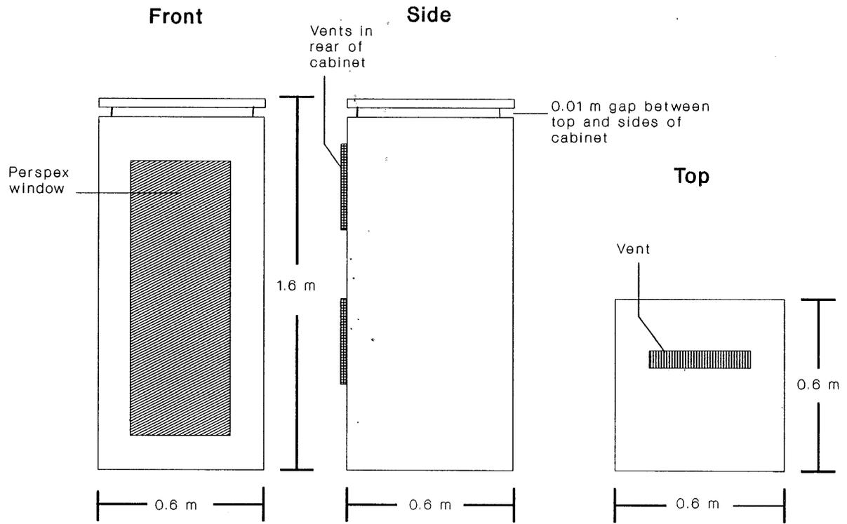
**Figure 9: Fire challenge inside an enclosed telecommunication cabinet**
