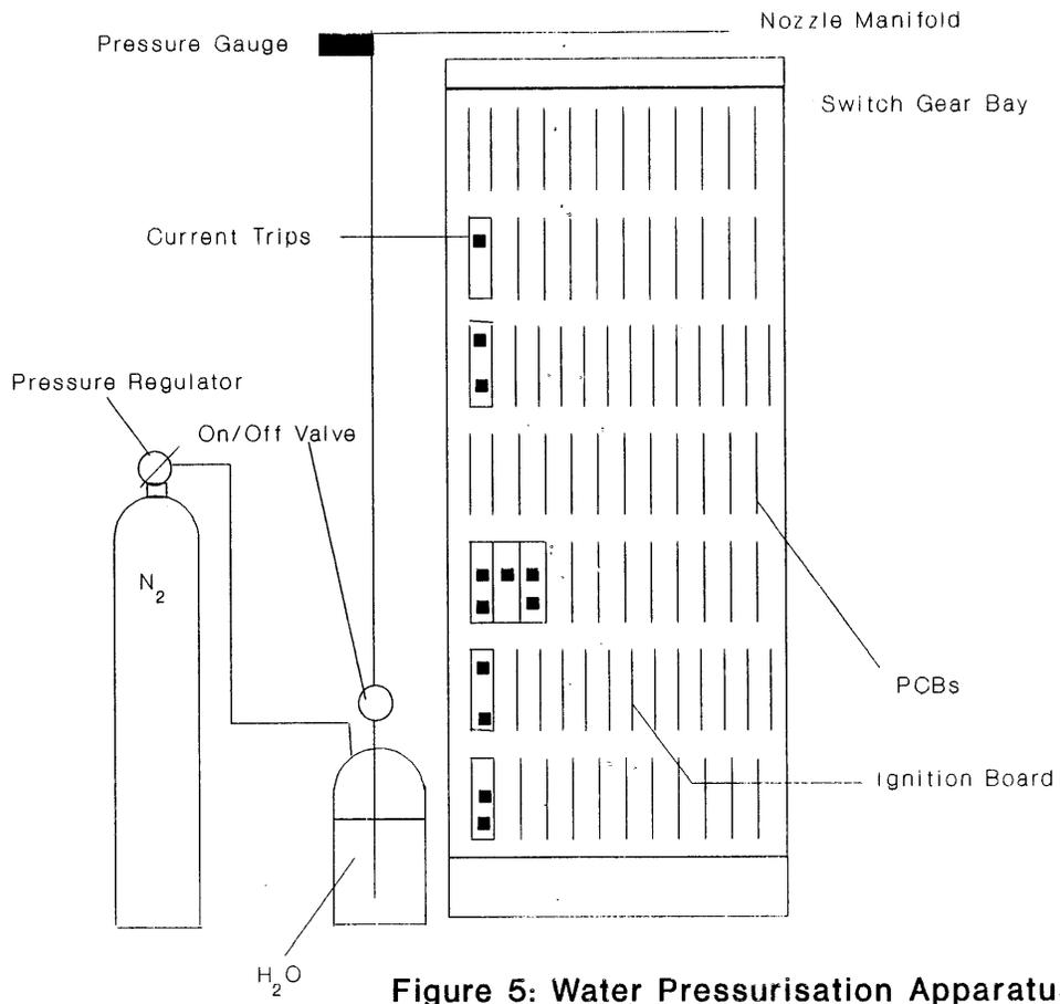
**Figure 5: Water Pressurisation Apparatus**
