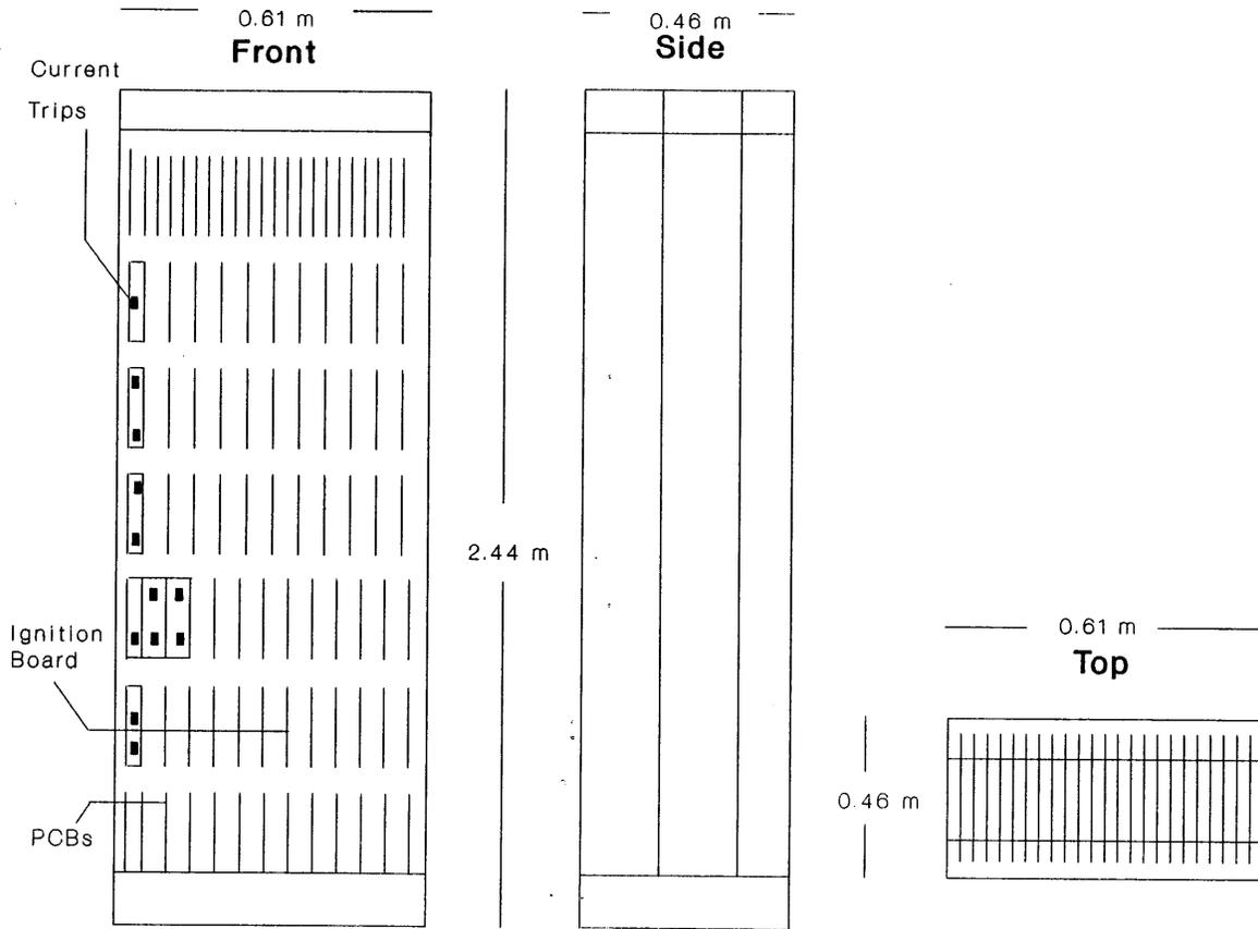
**Figure 1: A Typical Switch Gear Bay and Position of the Ignition Board**
