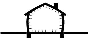
Figure 2. Pressure forces created by sudden pressure drop.
