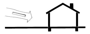
Figure 3. Impact forces created by missiles.
