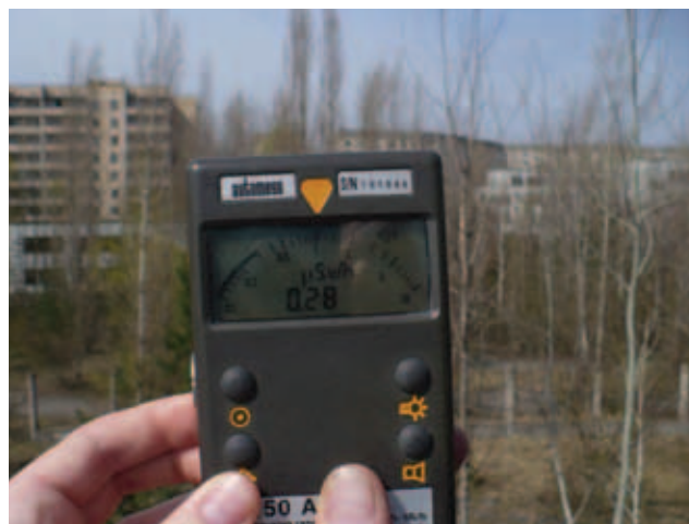
Figure 2. Measuring radiation on April 10, 2008 at a sport stadium downtown of Prypyat, about 4 km NW from Chernobyl reactor. The dose rate was 0.28 \mu\text{Sv/h} (2.5 mSv/year). Based on Fornalski (2009).
