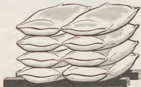
SUGAR SACKS STORED OFF THE FLOOR
