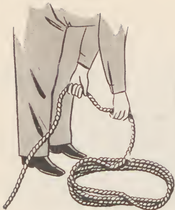
COILING ROPE ON GROUND
