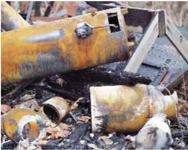
Water heater burned in residential fire caused by a gas leak.
