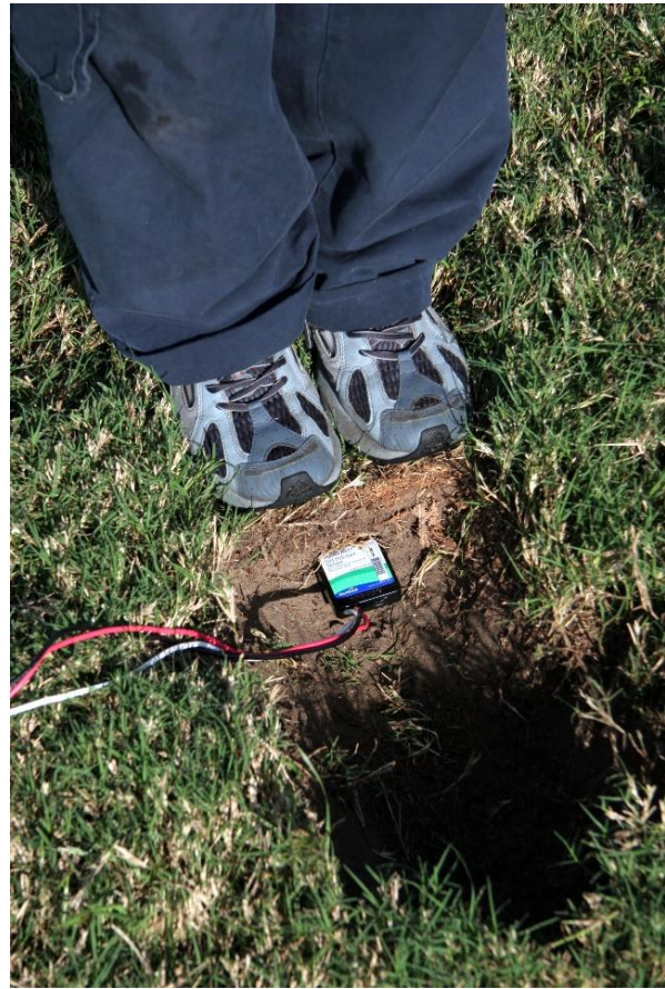
Figure 14. Compaction of soil around sensor to reduce void space and ensure adequate contact between SMS probe and soil
