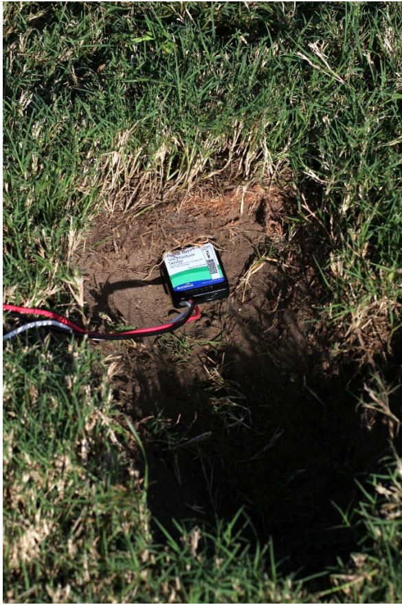
Figure 13. Wave guides of the probe completely inserted into the undisturbed wall of the hole
