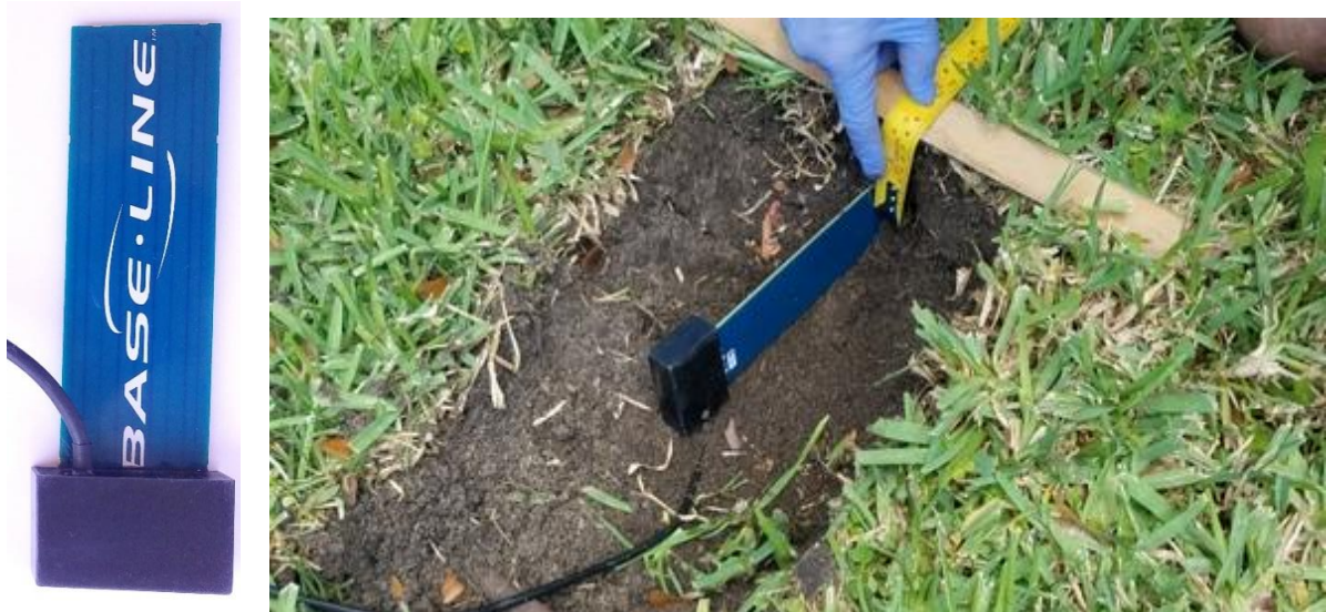
Figure 6. Sensor probe with encased wave guides been inserted within the root zone
