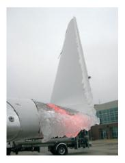
Accumulation of ice on aircraft is one of the most significant hazards to the safe and efficient operation of aircraft as it can reduce aircraft performance in a number of ways. Aircraft flying through cloud in sub-freezing temperatures are likely to experience some degree of icing.
