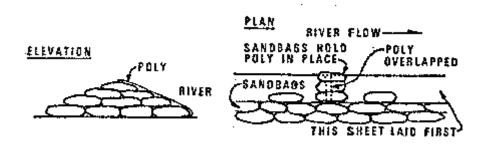
Polyethylene (plastic) comes in rolls 20 ft wide by 100 ft long. It is used to wrap sandbag levees to prevent seepage. Plastic should be placed on downstream portion of levee first, then worked upstream with a two to three foot overlap. Plastic is held in place with sandbag.
