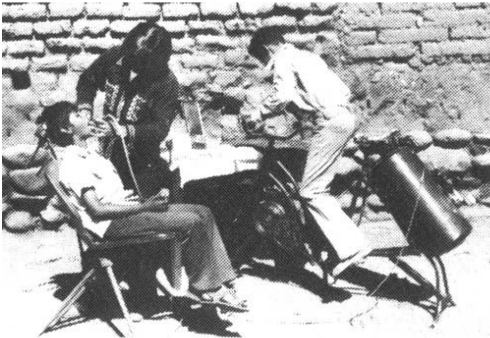
Village dental workers in the mountains of western Mexico use bicycle power to make compressed air, which runs a high-speed drill.
