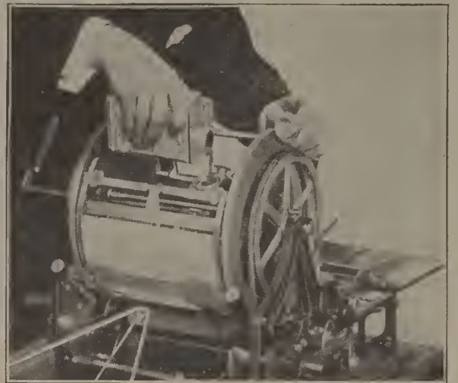
Proper method of filling the Ink Fountain
